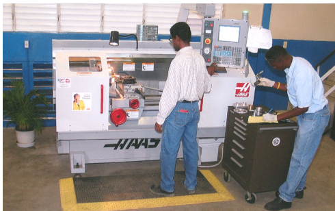
Using a part drawing to create a program for the CNC Lathe.
