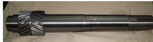
Herringbone gear-shaft for large overhead crane made on the CNC Milling Machine
