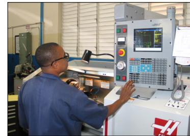
Manufacturing Associate shown programming the CNC Lathe
